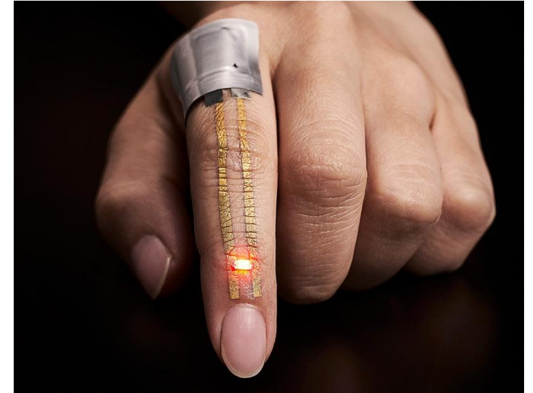
Index finger with gold nanomesh conductor
